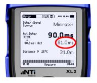
Now play the Delay signal from the MR-PRO through the front left PA speaker only. Remain at the audience position closest to the delay speaker. Add 15 ms to the delay difference shown on the XL2 (81 ms + 15 ms = 96 ms in this example), and apply this delay value to the delay speakers. Assuming the speaker layout is symmetrical, apply the same value to the right delay speakers, or measure again on the right.
