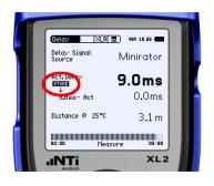
Play the Delay signal from the MR-PRO through the left delay speaker only. Stand at the audience position closest to the delay speaker and press the XL2 Delay STORE function. This sets your zero point.
