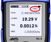
At the same point in the signal path, plug the XL2 into the up-line section of the path (from the mic or instrument). Select RMS/THD, create a sound at the source (ask the guitarist to play or gently tap the microphone) and check that the up-line signal is balanced. Press the speaker button on the XL2 and listen for the hum through the XL2 internal speaker.
