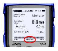
Play the DELAYTEST signal from the MR-PRO connected directly to the XL2 in order to synchronize the two instruments. When sychronised, the XL2 shows that you are now ready to measure the delay with the word "Measure". You now have 5 minutes to measure the delay before another synchronization is required.
