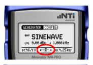
Plug the MR-PRO into the down-line section of the path (towards the mixer). Select 1kHz SINEWAVE and check that the down-line signal is balanced, because a missing screen on the cable or an unbalanced line can often cause the hum.
