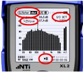
Select SLMeter RTA on the XL2, measuring LZSlive. Select 1/3 Octave resolution as this gives you 31 bands of resolution, matching most traditional equalizers. Position the XL2 microphone at the nearest audience position in front of the left speakers. When you are satisfied that the frequency response of the left PA has no significant spikes or dips, press pause on the XL2 to freeze the spectrum reading from the left PA.
